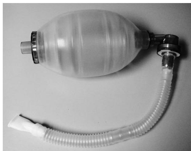
Fig. 6. Manual insufflator, consisting of a resuscitator bag, a one-way valve, a flexible tube, and a mouthpiece.
